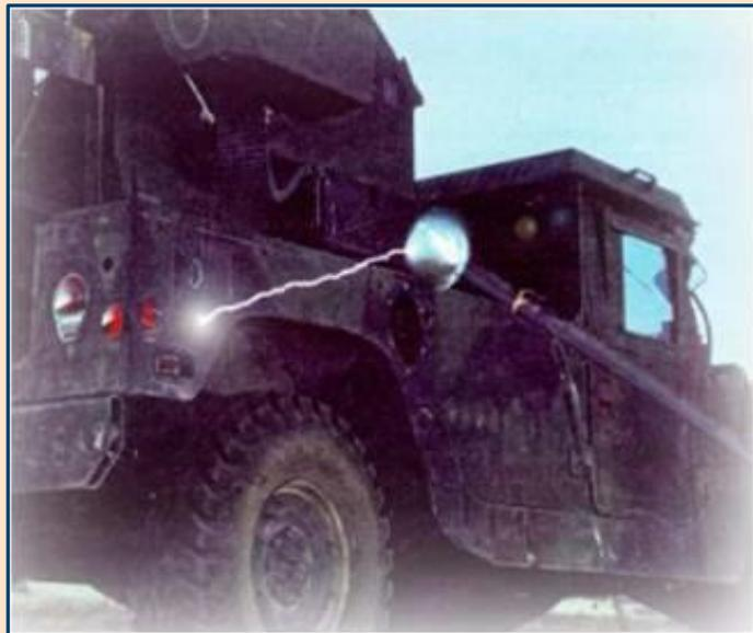
**ELECTROSTATIC DISCHARGE (ESD) FACILITY:** Electrostatic discharge (ESD), or static electricity, can be potentially devastating to sensitive electronics. To ensure that weapon systems are hardened against damage from ESD, we perform both personnel-level (25,000 volts direct current) and helicopter-level (350,000 VDC) ESD testing.
