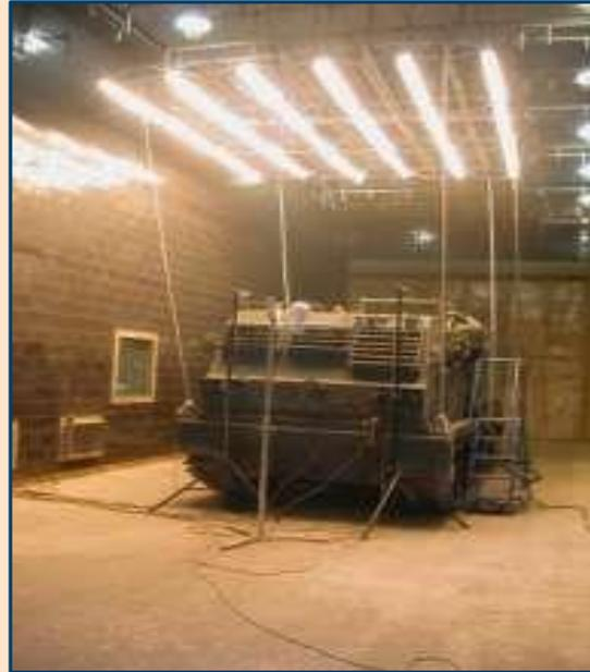
**RADIATION CORRELATION LABORATORY (RCL):** provides gamma environments (Cobalt-60 and Cesium-137) for realistic evaluation of performance of radiation detectors and sensors. It is also used to determine shielding characteristics of vehicles.
