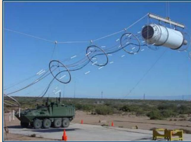
**GAMMA RADIATION FACILITY (GRF):** The GRF is designed to provide the total gamma dose and residual gamma dose environments needed for nuclear effects testing of virtually any size item.
