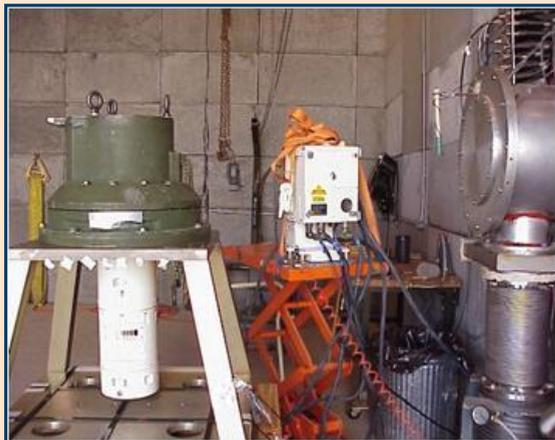
**RELATIVISTIC ELECTRON BEAM ACCELERATOR (REBA):** The REBA (1.9MeV) and PI 538 (4.2 MeV) is a high-energy, pulse, field emission electron beam or Bremsstrahlung x-ray source. These simulators produce the gamma dose rate environments of a nuclear weapon detonation.
