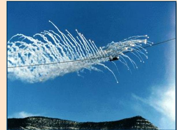
The ACR can be stationary or dynamic. Dynamic gravity rolls up to 120 knots and rocket boosted up to 240 knots
